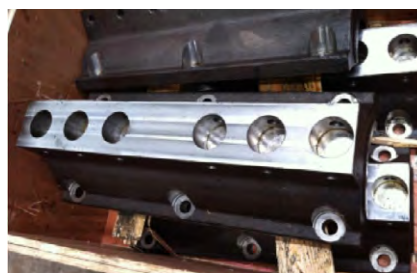
Ash Crusher Roll Supports
